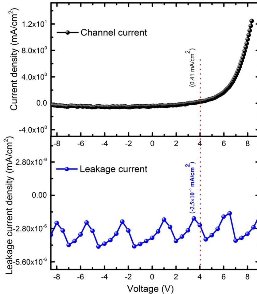
**Fig. S4.** A leakage current density test on the 20 nm-thick SiO<sub>2</sub> dielectric layer was conducted by scanning the gate bias from -8 to 8 V for four cycles. A typical plot of the leakage current density as a function of gate voltage is shown in the lower panel. A comparison of the channel current density (in the upper panel) with the leakage current density (in the lower panel) is presented with the values of current density being labeled at the gate bias of 4 V.
