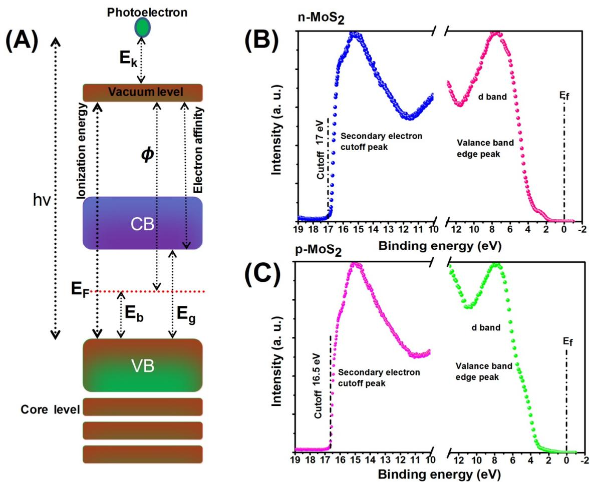
**Fig. S1.** (A) Schematic representation of the energy diagram related with the observations by UPS spectroscopy.  $E_b$ : binding energy,  $E_f$ : Fermi energy,  $E_g$ : band gap energy,  $E_k$ : kinetic energy of an escaped electron,  $\phi$ : work function. (B–C) The UPS spectra of (B) n-MoS<sub>2</sub> and (C) p-MoS<sub>2</sub> were observed, where the binding energies at the cutoff edge are determined to be 17 eV and 16.5 eV, respectively.
