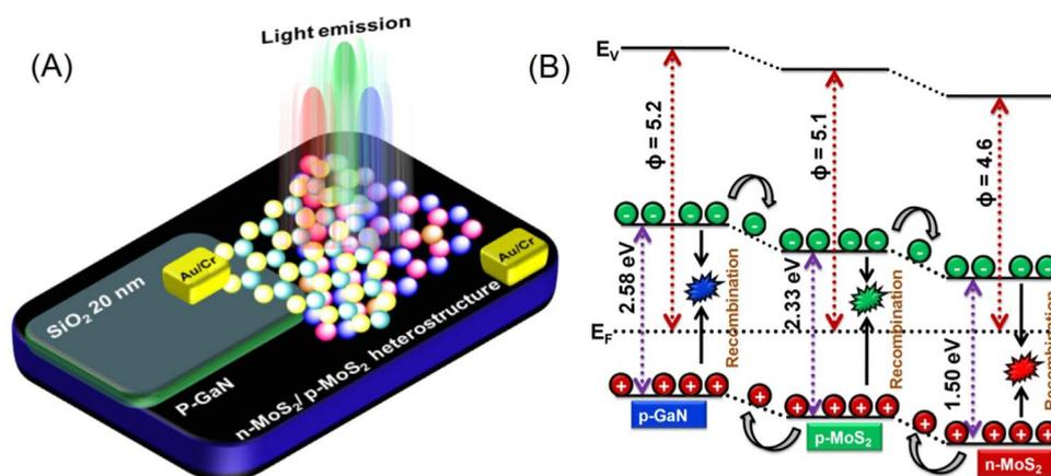
Fig. 4. A WLED device with the 4-L n-MoS<sub>2</sub>/p-MoS<sub>2</sub>/p-GaN heterostructure. (A) Schematic illustration of the WLED device constructed by three emitters in the n-MoS<sub>2</sub>/p-MoS<sub>2</sub>/p-GaN. (B) The band alignment of the vertically stacked n-MoS<sub>2</sub>/p-MoS<sub>2</sub>/p-GaN heterostructure with the band energies obtained from the UPS analysis.
